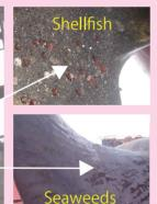
Propeller surface is roughened by adhesion of shellfish and seaweed. By these, propeller performance deteriorates.
